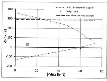
**DESIGN LOADS FALL WITHIN THE LIMITS** OF THE INTERACTION DIAGRAM, THEREFORE, USE (8) # VERTICAL BARS IN COLUMN.
